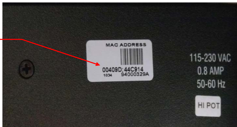
Figure 10: MAC address label on serial server
