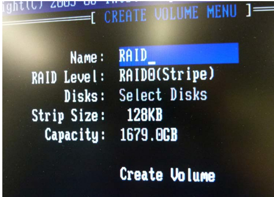
Figure 48: Create RAID volume
