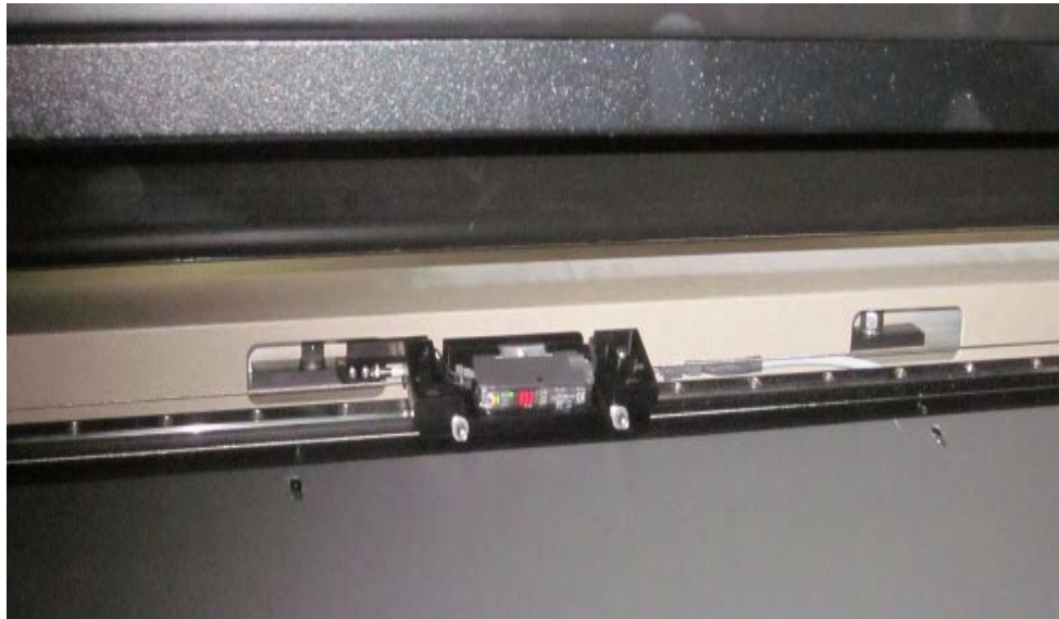
Figure 27: Tick mark sensor for double-sided printing
