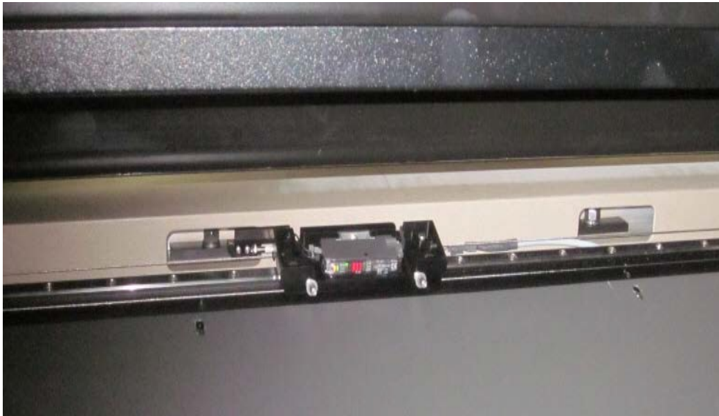
Figure 38: Tick mark sensor for double-sided printing
