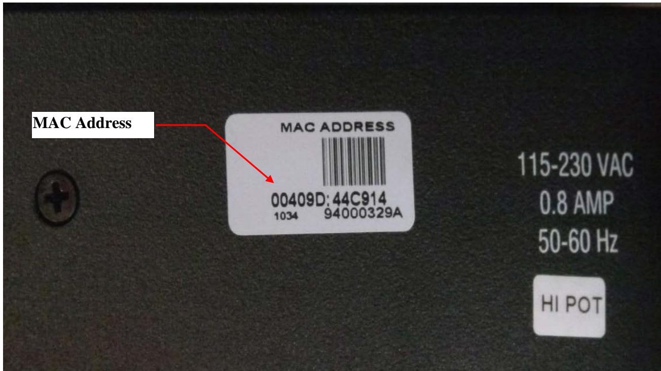
Figure 52: MAC address label on serial server
