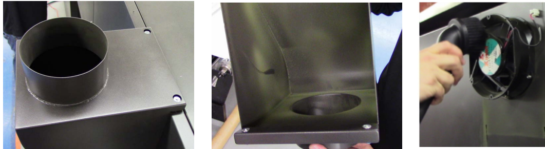
Figure 9-5 Metal Exhaust Vent Housing (Left and Middle) and Vacuuming Exhaust Fan (Right)
