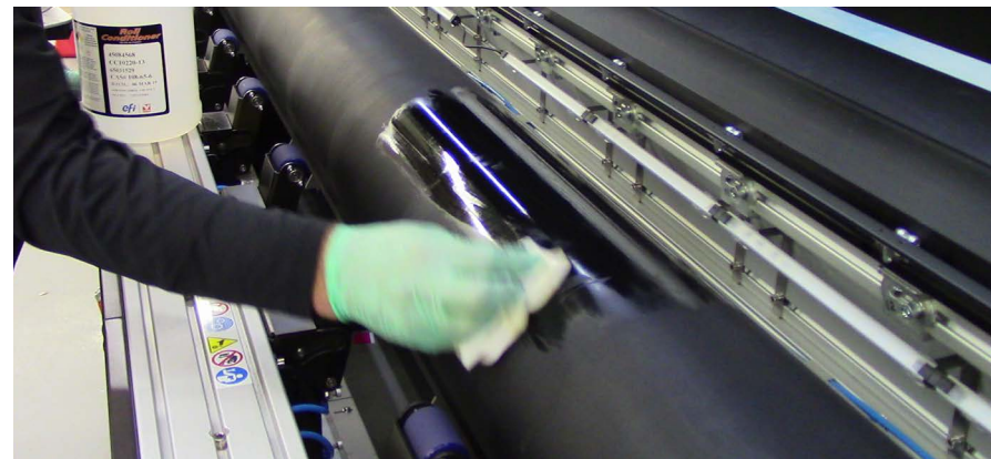
Figure 7-2 Cleaning Tension roller
