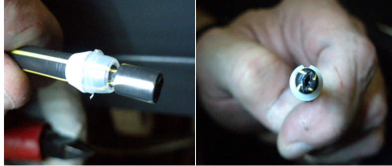
Figure 2-55: Tubing damaged due to over-tightening fittings
