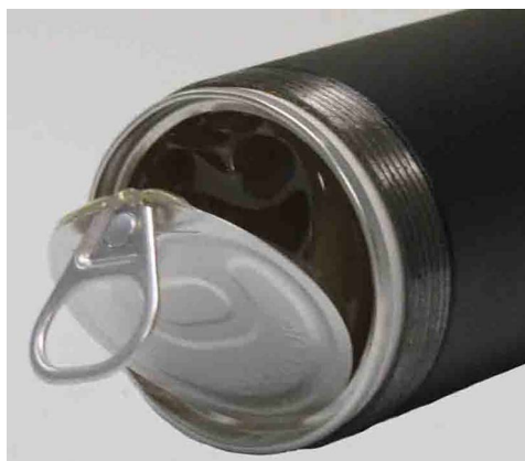
Figure 2-61: Grease tube inserted into grease gun with cap partially removed
