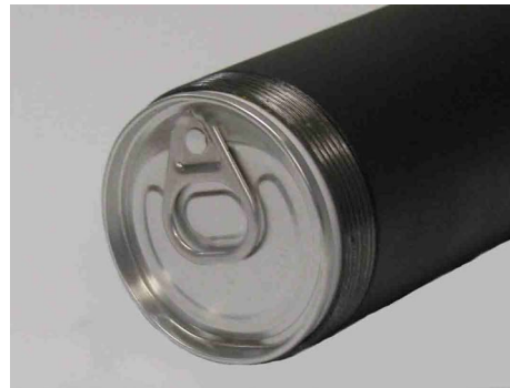
Figure 2-60: Grease tube inserted into grease gun metal tube
