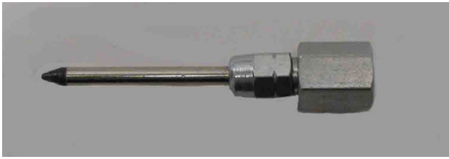
Figure 2-75: Bearing grease tip
