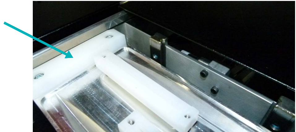
Figure 2-74: Wear strips on Vacuum Purge Tray
