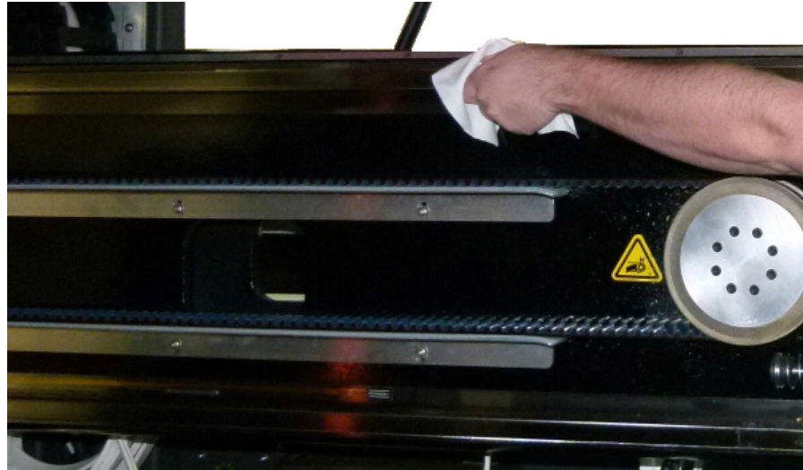
Figure 2-12: Cleaning the carriage rail ends
