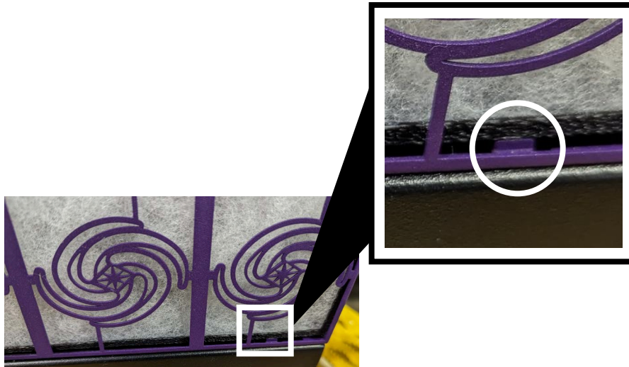
Figure 5-4 New Filter Not Seated in Holding Tab
