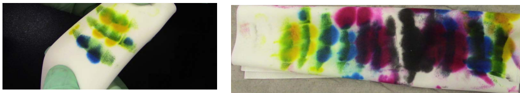
Figure 3-7 Advancing to clean portion of wipe, Left, and discarded wipe, Right
