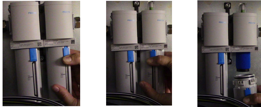
Figure 6-10 Removing filter cover
