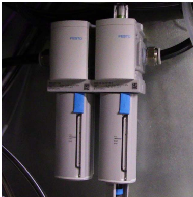
Figure 6-9 Nitrogen Filter Packs, Left, and Filter Status Viewing Window, right
