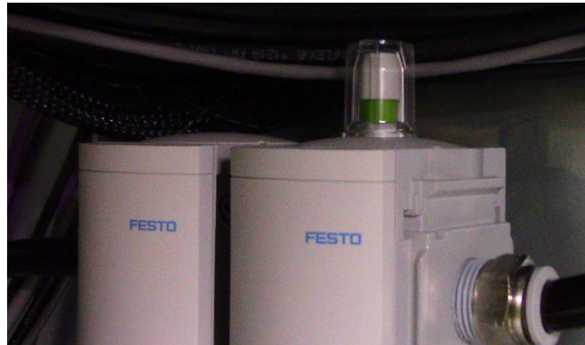
Figure 6-9 Nitrogen Filter Packs, Left, and Filter Status Viewing Window, right
