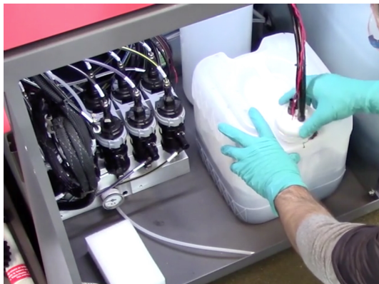
Figure 4-19 Unscrew Waste Container Cover
