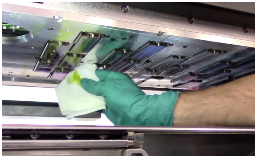
Figure 3-4 Wipe Perimeter of Print Head Plate and Between Print Heads
