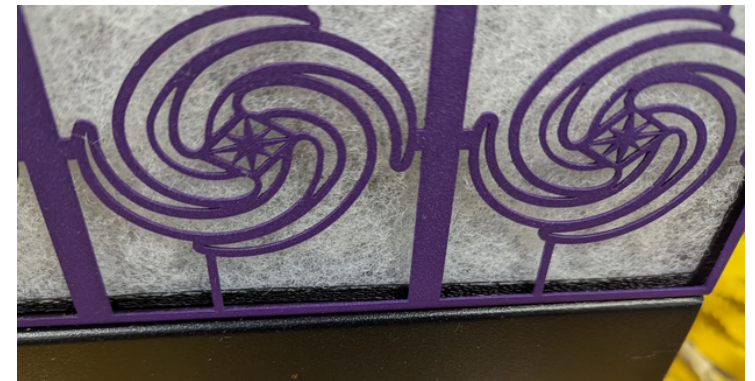
Figure 5-5 Correctly Seated Filter
