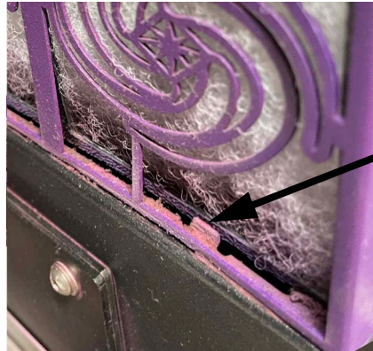
Figure 5-3 Badly Seated Filters Are Ineffective
