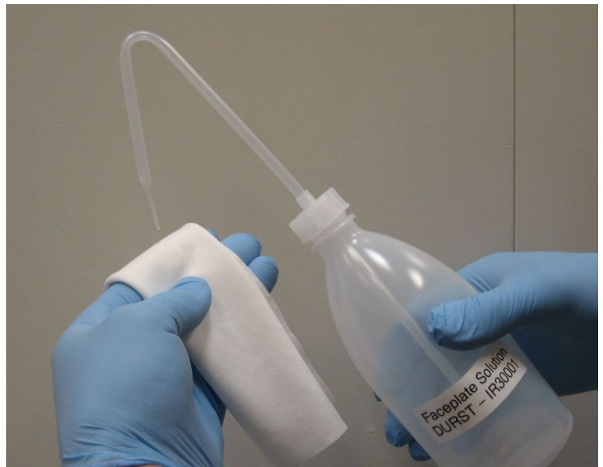
Fig. 77 Saturating cleaning cloth with cleaning solution
