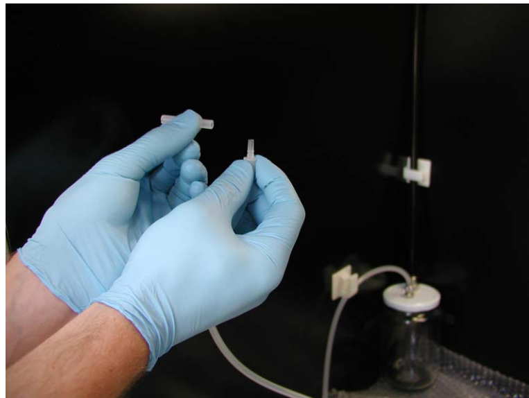
Fig. 93 Placing silicone tube on the vacuum hose.
