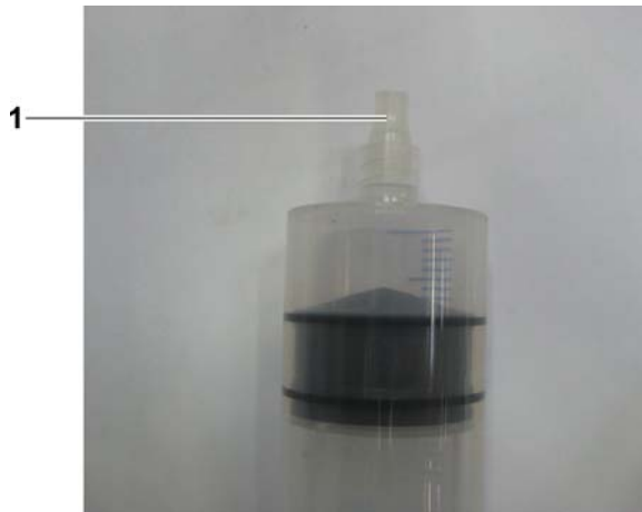
Fig. 96 Placing silicone tube on the tip of the syringe
