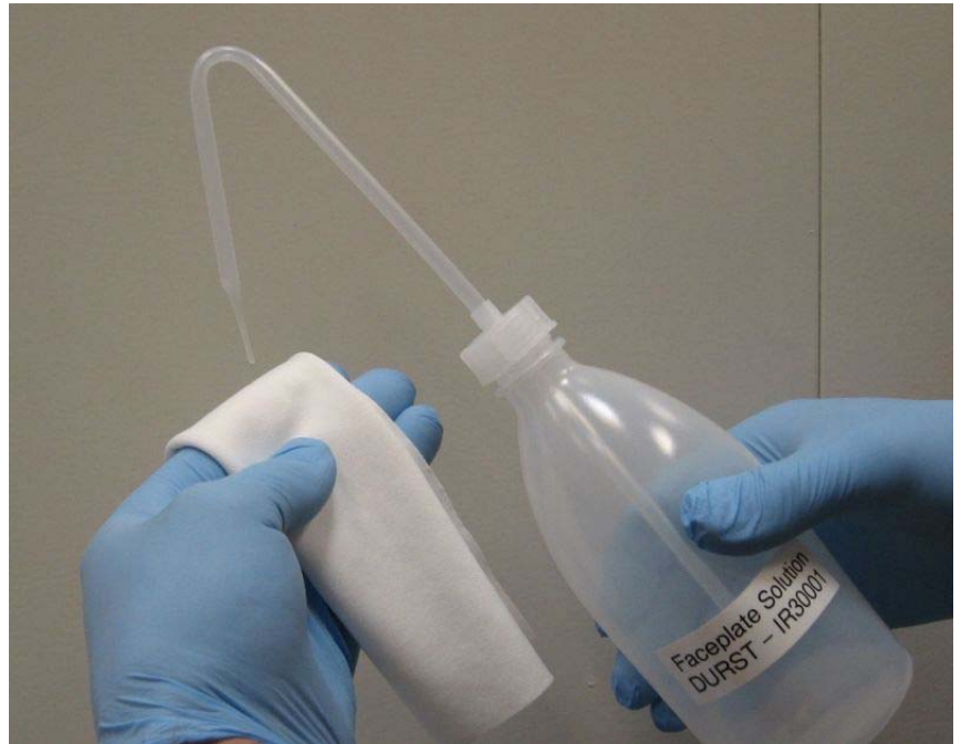
Fig. 91 Saturating cleaning cloth with cleaning solution
