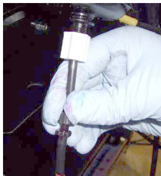
Fig. 86 Inserting new ink filter
