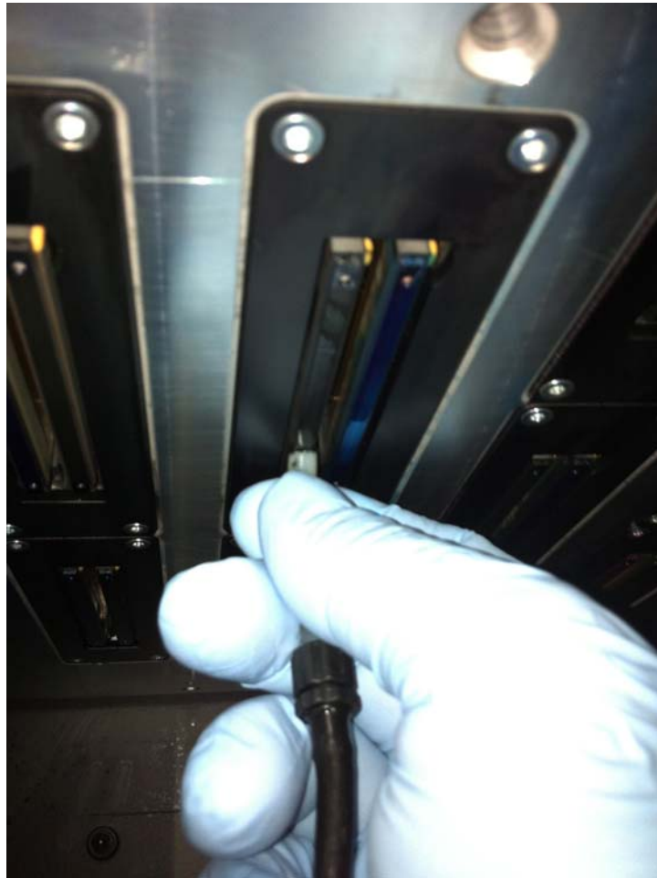
Fig. 95 Vacuuming out the print head
