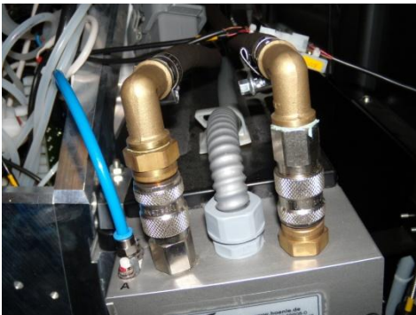
(hoses of water circulation must be connected)
