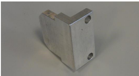
(bracket to protect the thermo switch in the lamp housing)
