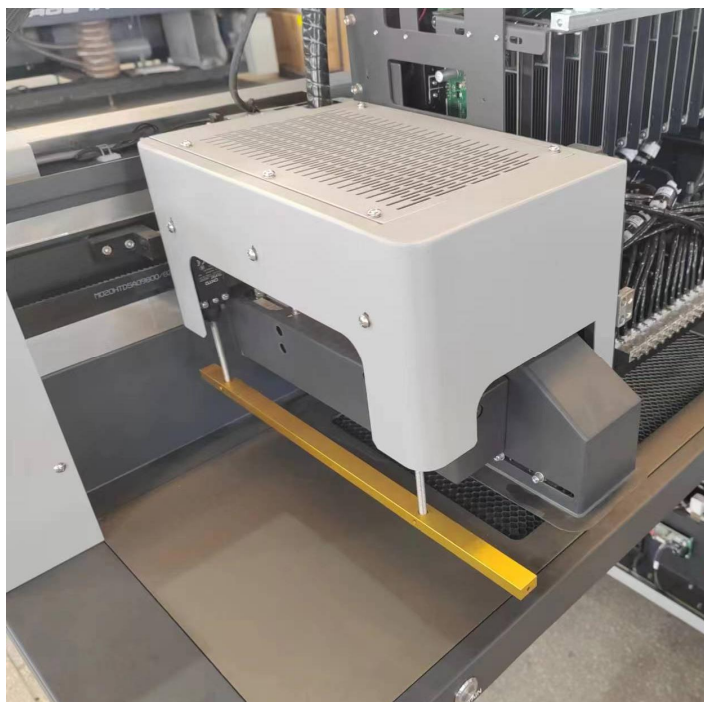
Fig. 207 Emergency stop anti-collision rod on both sides of carriage
