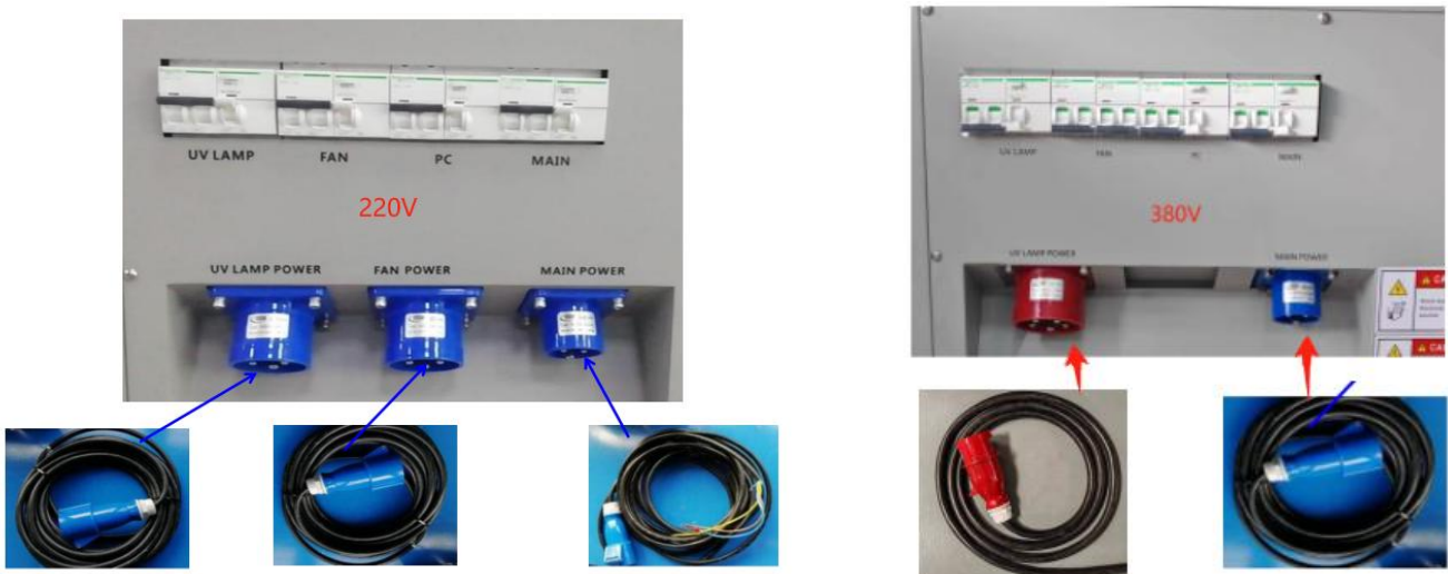
Fig. 33 AC Power connection of the hybrid printer
