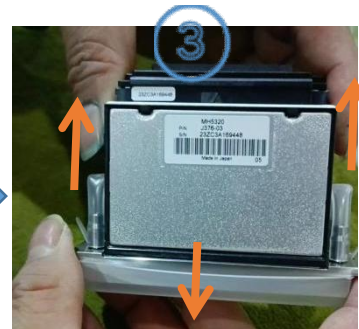
Remove the plug tube of the ink inlet and remove the protective cover for the nozzle surface.
