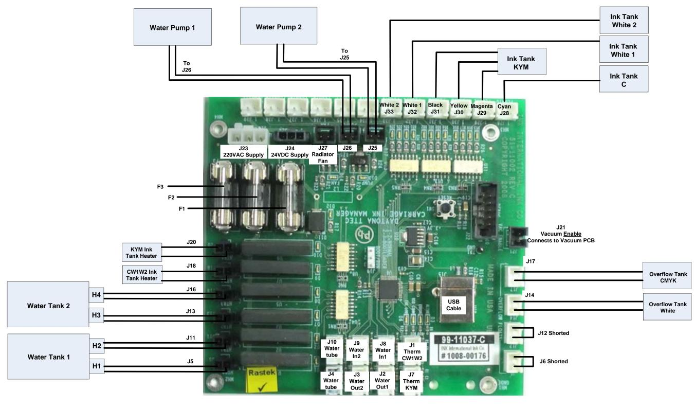
**NOTE:** Jumpers are required on J6 and J12 on all software versions. J4 and J10 thermistors have been removed on printer serial number T25 and above therefore a jumper will be required at J4 and J10. When installing version 3492 or greater software J4 and J10 thermistors can be removed and jumper installed at both connections.
