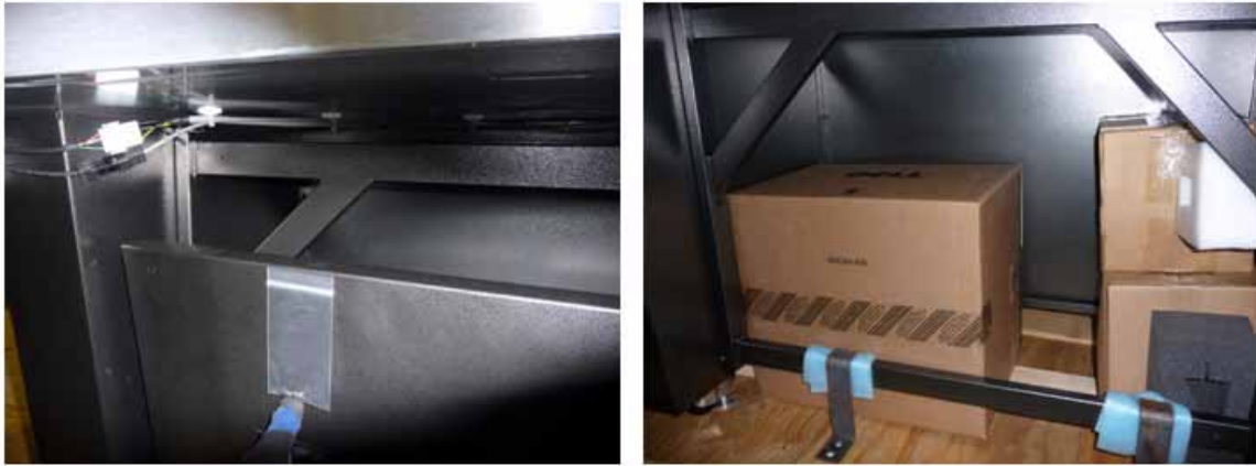
Figure 4-8: Removing Rear Panel
