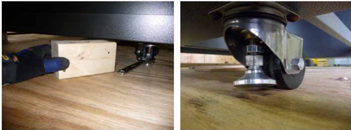
Figure 4-9: Printer feet and frame blocks
