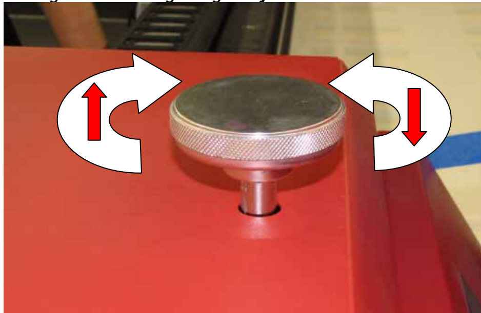
Figure 33: Carriage height adjustment knob directions
