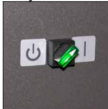
Figure 8: Auxiliary Power Switch – On position
