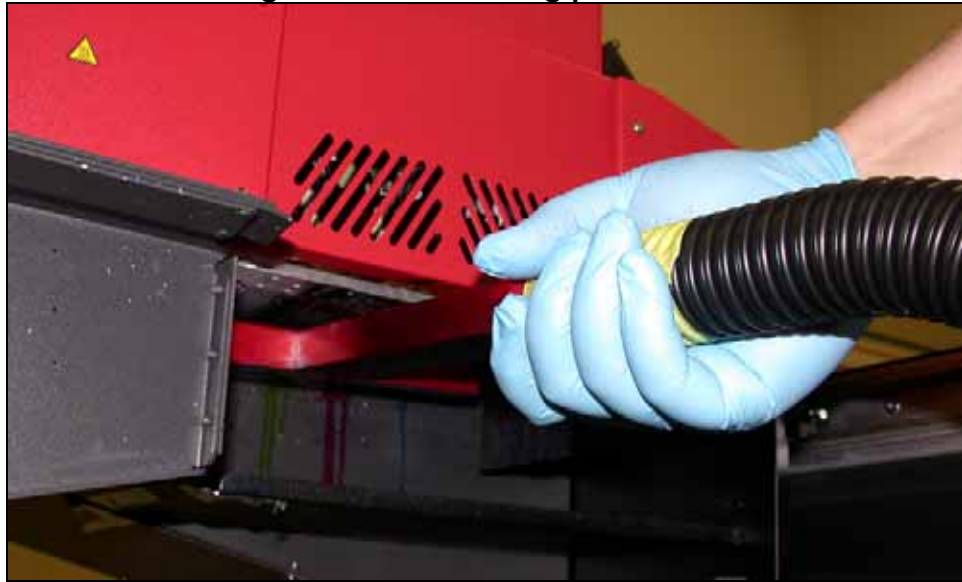
Figure 47: Vacuuming print heads
