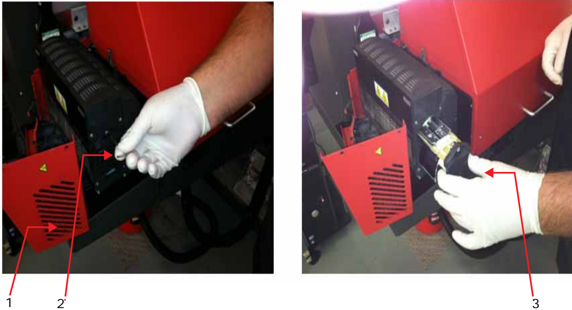
Figure 1-17: UV Bulb Base Removal
