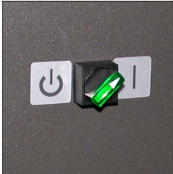
Figure 5: Auxiliary Power Switch – On position
